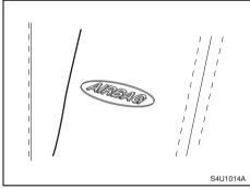
The words AIR BAG will appear on the side of the front seatback closest to the door, to indicate the presence of a side impact air bag.
